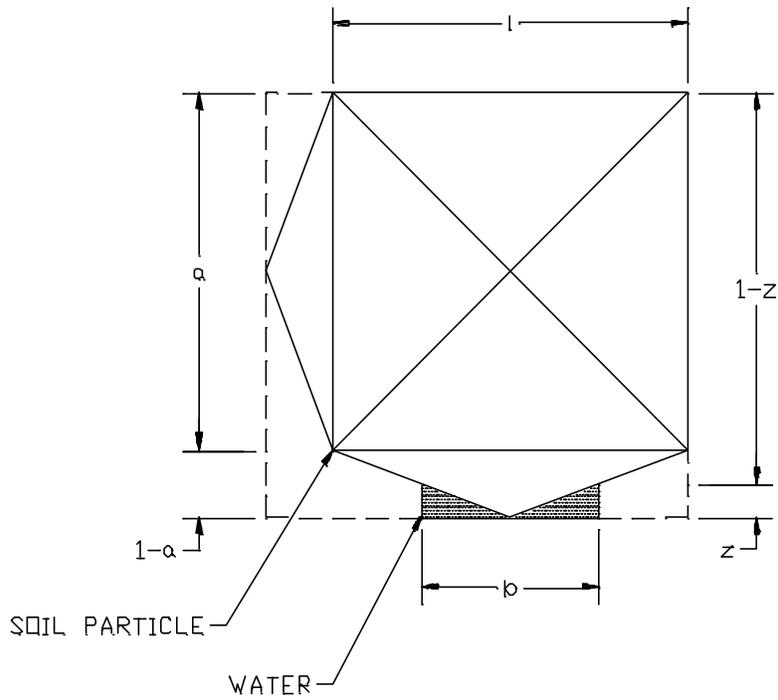
Figure 1: Idealized Soil Particle used in Gemant's Correlation (After Farouki [13]).
