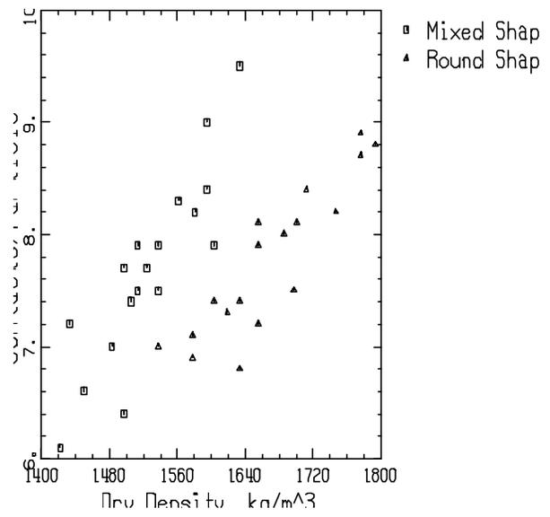
Figure 9: Number of Contacts/Particle vs. Dry Density for Mixed Shaped Particles ( $\square$ ) and Round Shaped Particles ( $\triangle$ )
