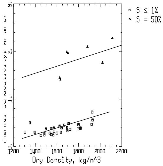
Figure 8: Thermal Conductivity vs. Dry Density for Unfrozen Sand at Two Saturation Levels:  $S \leq 1\%$  ( $\square$ ) and  $S = 50\%$  ( $\triangle$ )
